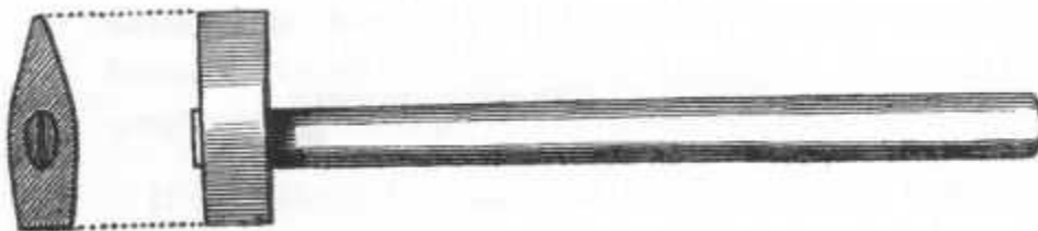
SKETCH 5: HAMMER FOR COLLECTING GEOLOGICAL SPECIMENS.
